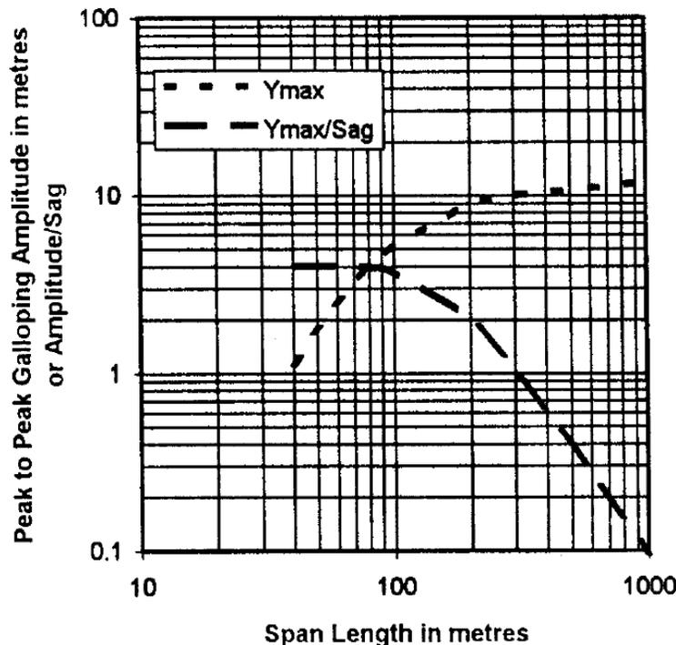
Figure 2 Observed Galloping Amplitude vs. Span Length
