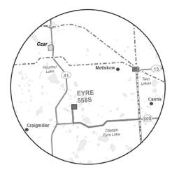
The Proposed Transmission Development Area indicated on the map above shows the approximate location of the proposed reinforcement. The proposed system reinforcement involves approximately 15 kilometres of single-circuit, 144 kV (144 000 volts) transmission line and a new 144 kV transmission substation, named Eyre 558S.
