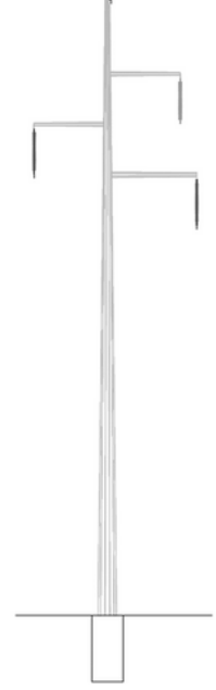
240kV Single Circuit Steel Monopole Typical Tangent Structure Height range approximately 30m – 40m
