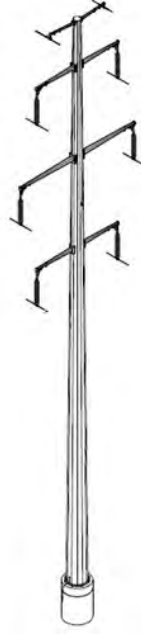
240kV Double Circuit Steel Monopole Typical Tangent Structure Height range approximately 30m – 45m
