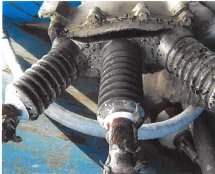
Figure 13 Failure of Pothhead due to Insulation Compound Leak (Kennedale)
