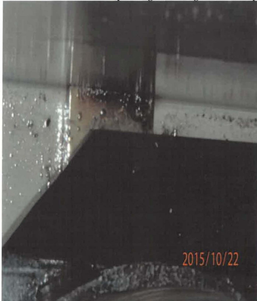
Figure 2 Kennedale Tx1 - Carbon build up and signs of arcing on reactor support
