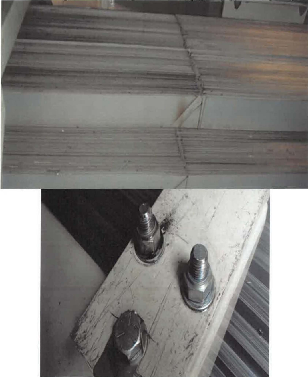
Figure 3 Kennedale Tx1 - Signs of overheating on the core top yoke (top) and tie plate (bottom)
