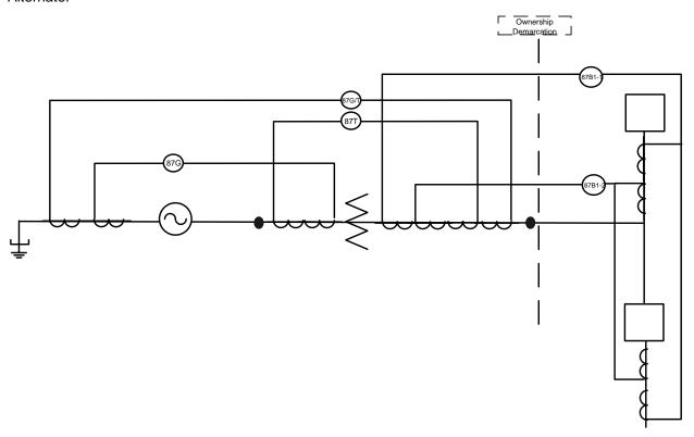
Typically one (1) of the protection systems for the generating unit provides one hundred (100%) percent stator ground fault protection.
