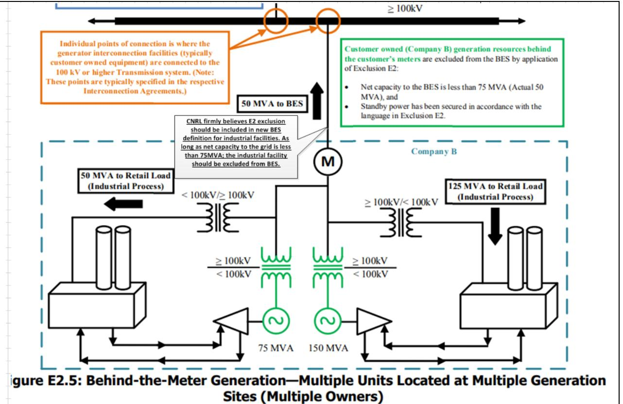
Figure E2.5: Behind-the-Meter Generation—Multiple Units Located at Multiple Generation Sites (Multiple Owners)
