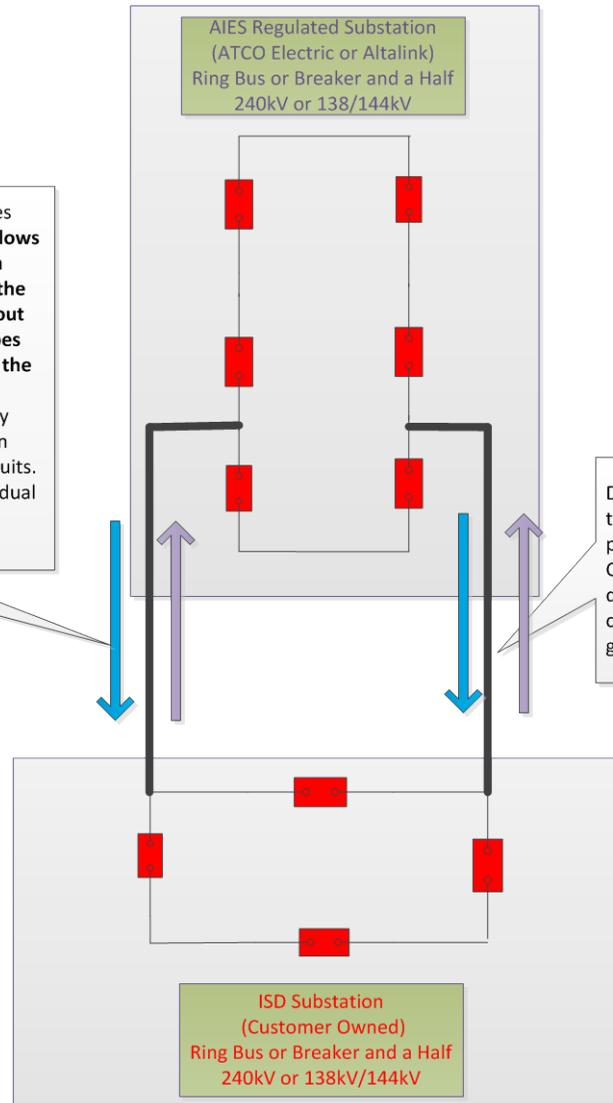
Dual Circuit connection from ISD to AIES is purely for redundancy purposes. CNRL's position is that type of dual circuit connection is radial connection to the wider AIES grid.
