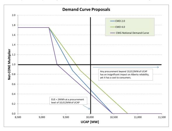
The purple, or left-most curve, represents a more reasonable demand curve that achieves target availability at equilibrium and was submitted by the CWG in response to CMD 3.0. In light of the analysis that shows that at 10,012 MW of UCAP the EUE is at 2 MWh, it should be considered whether an improvement of this curve would be to reduce the width of the foot.
