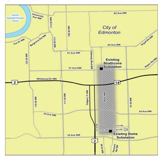
The shaded area on the map indicates the approximate location of the proposed 72 kV transmission line. The black squares on the map indicate the approximate location of the Strathcona substation (SE-5-16-52-24-W4) and Dome substation (SE-3-4-52-24-W4).
