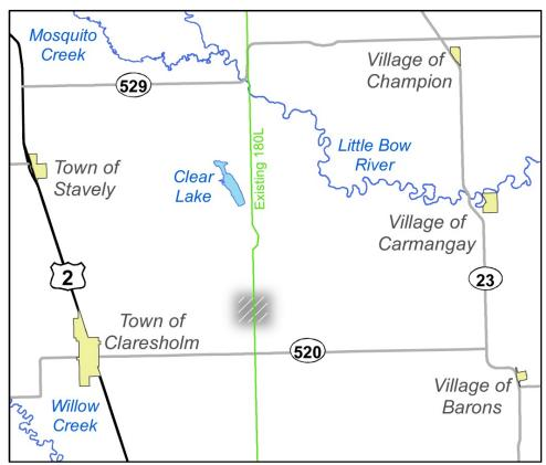
The shaded area on the map indicates the approximate location of the proposed transmission developments, including the 138 kV transmission line. The specific transmission facilities may extend beyond the shaded area shown.
